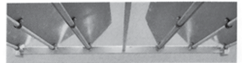
Unlike all others, the roll-damping function engages immediately (blades open slightly or fully).
